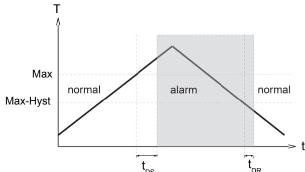
In the non-inverted (standard) model, while in the normal state the switching output is at the level of the supply voltage; in the alarm state it is at 0 V, so that a wire break would also display as an alarm state at the signal receiver. Optionally, an inverted switching output can also be provided, i.e. in the normal state the output is at 0 V, and in the alarm state it is at the level of the supply voltage.
