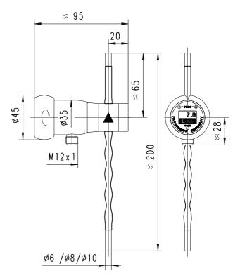
A spacer between the electronics head and the medium-contact measurement tube provides thermal decoupling between the two units. The media temperature may be raised for 45 min. to 130  $^{\circ}$ C.
